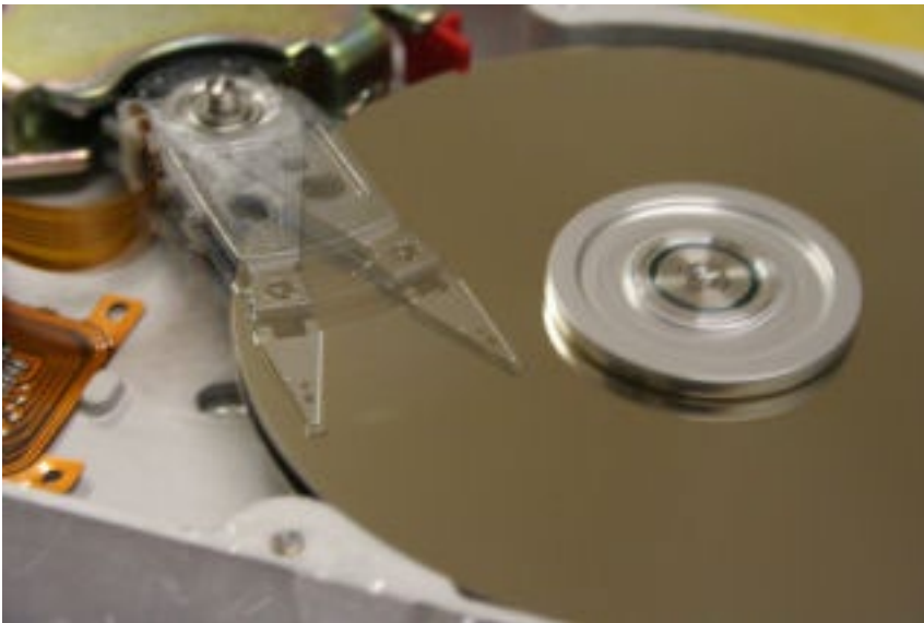
Internal view of a hard drive in operation. The arm appears blurred due to its rapid movement. Photo courtesy of Michael Blessenohl
